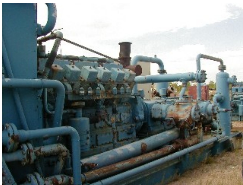
Figure 22. A hydrogen compressor that can be used to boost the pressure from the production plant to a specified pipeline pressure.
