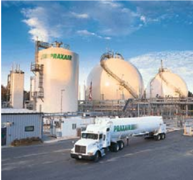
Figure 16. A tractor-trailer that can deliver liquid hydrogen to a forecourt station (photo downloaded from the Praxair website).
