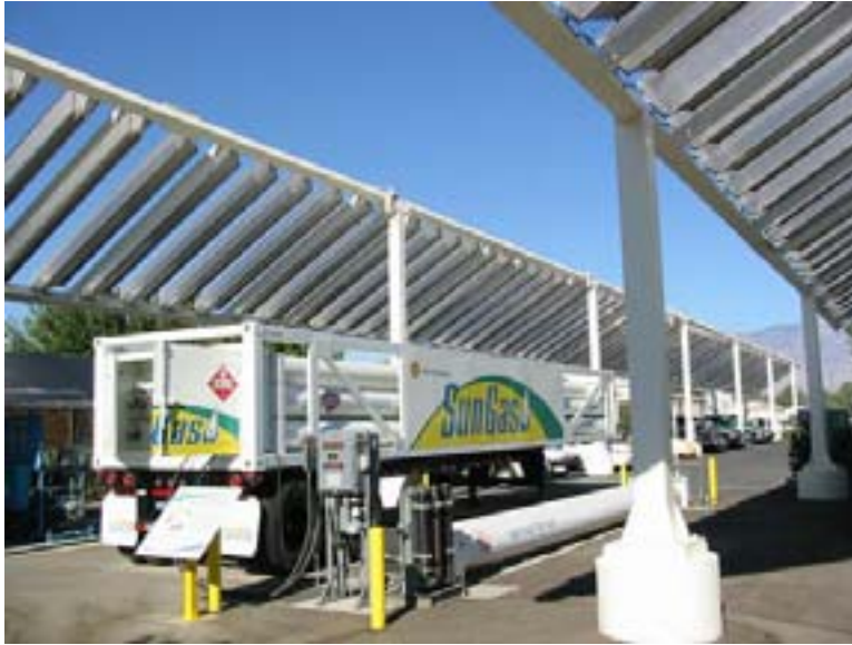
Figure 14. Picture of a current technology tube trailer (photo downloaded from NREL PhotoPix library).
