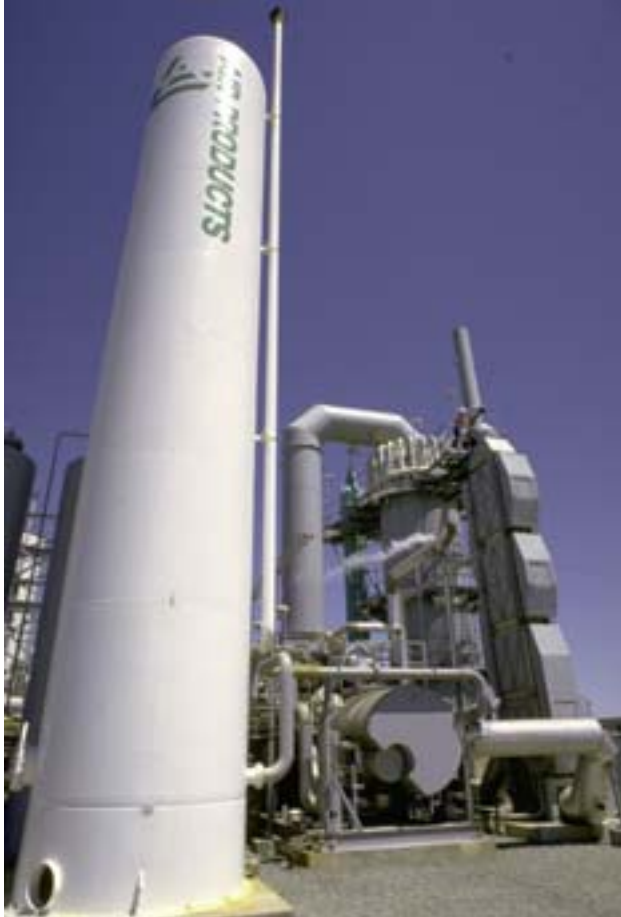
Figure 17. An Air Products hydrogen liquefaction facility in Sacramento, CA (photo courtesy of Air Products and Chemical's website, at www.airproducts.com ).
